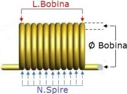
CALCOLO INDUTTANZA BOBINA MONOSTRATO IN ARIA by IU5HIV [Back](#)
